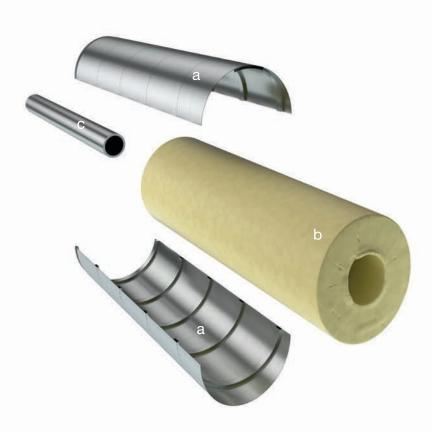
A bonded pipe system is created. The system performance is superior to conventionally insulated pipes, because the carrier pipe encased by the insulation foam in a metal jacket acts as one strong unit better able to resist external forces. So sliding supports can be mounted on the outside jacket which is not possible if traditional insulation is specified.
