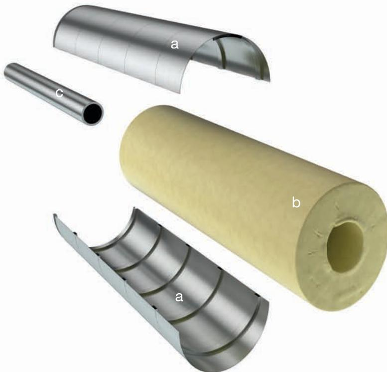
A **bonded pipe system** is created. The system performance is superior to conventionally insulated pipes, because the carrier pipe encased by the insulation foam in a metal jacket acts as one strong unit better able to resist external forces. So sliding supports can be mounted on the outside jacket which is not possible if traditional insulation is specified.
